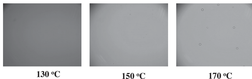
Figure 4. Optical microscopic pictures of PCPO25 according to annealing temperature after 10 min annealing at the test temperature.
